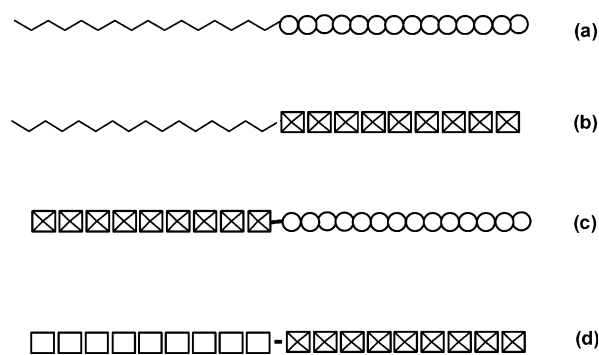
Scheme 1. Schematic representation of diverse types of stimuli-sensitive macro-surfactants: (a) hydrophilic and hydrophobic blocks fixed (classical structure), (b) hydrophilic block stimuli-sensitive, (c) hydrophobic block stimuli-sensitive, (d) both blocks stimuli-sensitive (OOO, hydrophilic segment; \sim\sim\sim\sim\sim\sim\sim\sim , hydrophobic segment; \square\square\square , \boxtimes\boxtimes\boxtimes , switchable segments).
